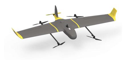
The Fujin is capable of Vertical Take-off and Landing operations while having all the capabilities of a heavy lifting fixed-wing plane. It combines the power-saving capabilities of a fixed-wing aircraft with the precision of a drone and delivers a longer flight time.
